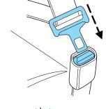
• Grasp the shoulder portion and pull downward until the entire belt is pulled out.
